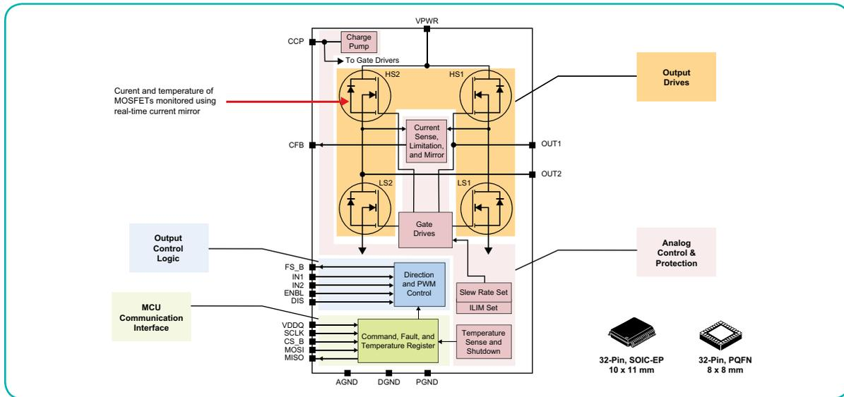
Figure 3. MC33HB2000 & MC33HB2001 architecture and packaging
