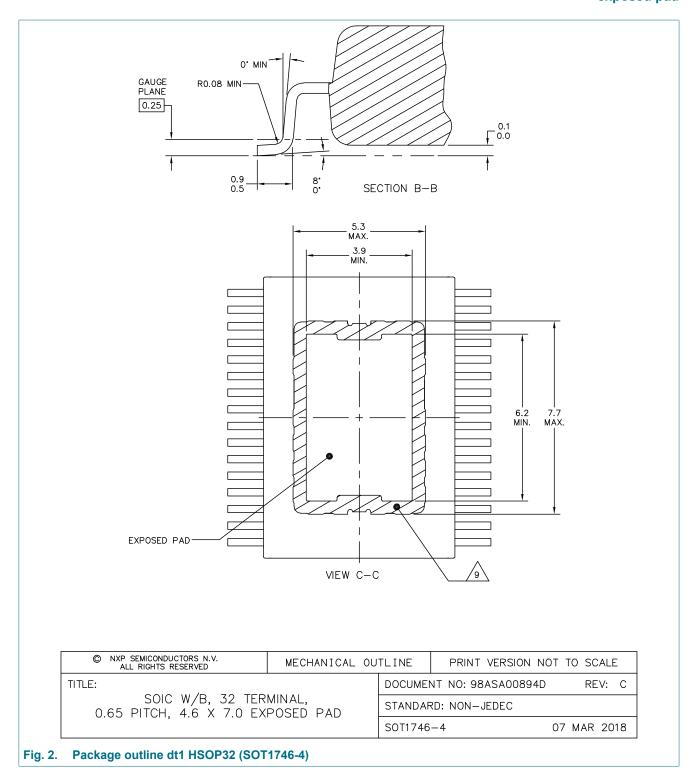
HSOP32, plastic, thermal enhanced small outline package; 32 terminals; 0.65 mm pitch; 4.6 mm x 7 mm exposed pad
