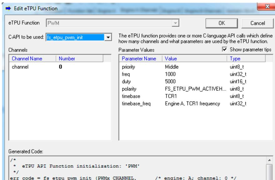
The following source code is generated in C-programming language for the initialization function of PWM signal initialization there, as shown in Listing 1.
