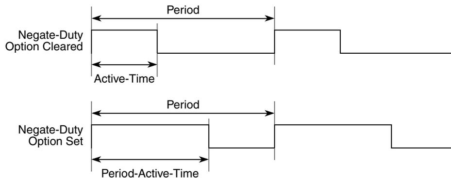
Figure 11. Effect of the Negate-Duty Option on Edge-aligned PWM Signals
