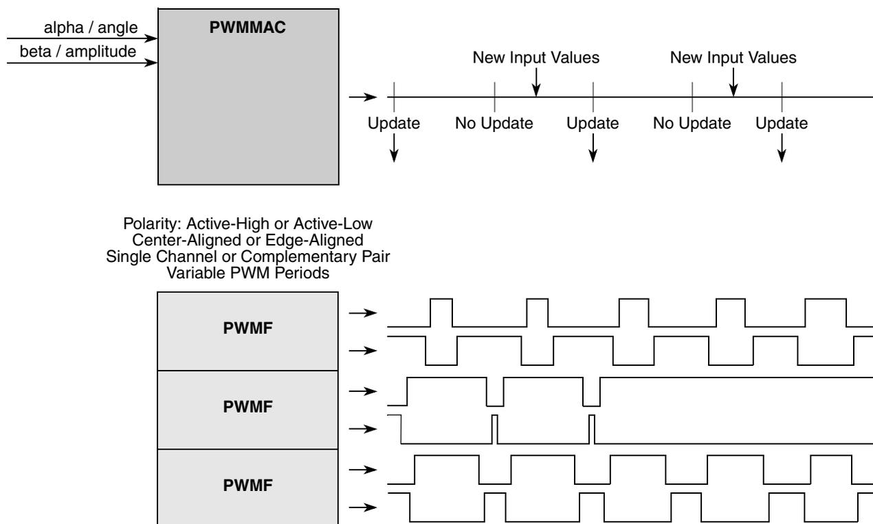
Figure 1. Functionality of PWMMAC+PWMF
