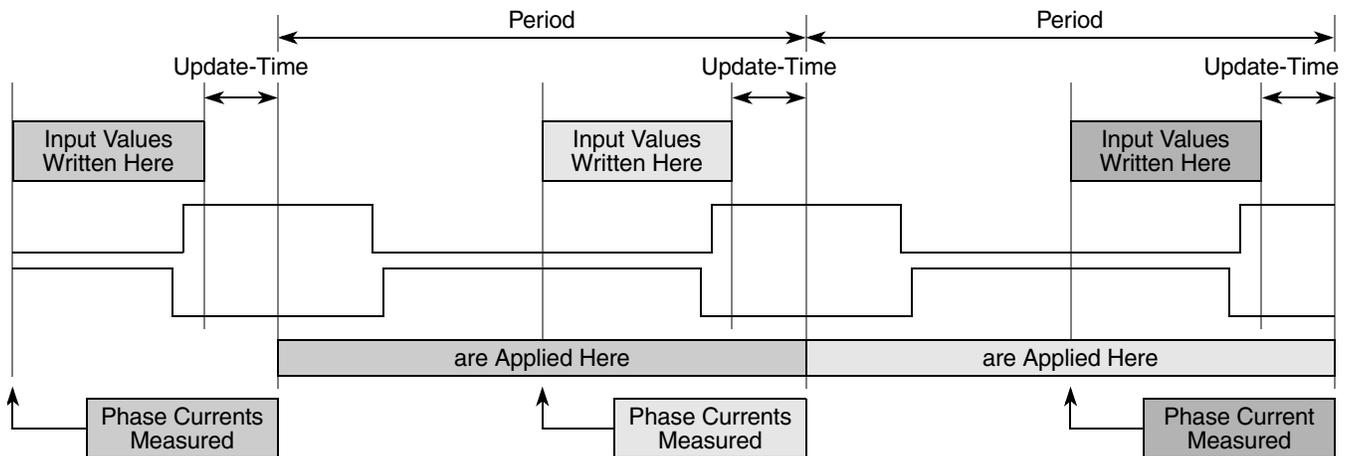
**Figure 21. Timing Corresponding to the Configuration on Figure 20**
