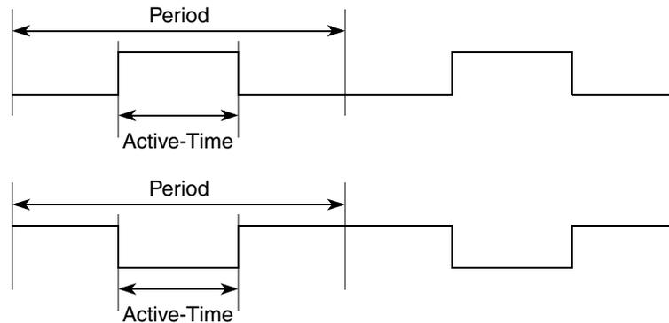
Figure 10. Example of PWM Signals of Different Polarity
