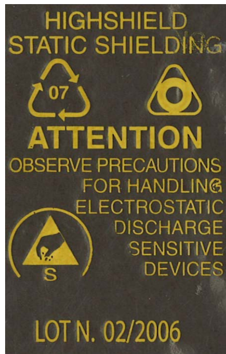
Fig 15. Typical warning label of ESD sensitive devices
